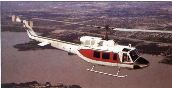
The Model 212 Twin Two-Twelve has almost the same structure as the UH-1H and related models, but is powered by the PT6T-3B engine which has two separate power sections, giving twin-engine safety. The Twin Two-Twelve commercial version, as seen here, was certificated in 1970 to carry a 5,000-lb (2268-kg) load.
