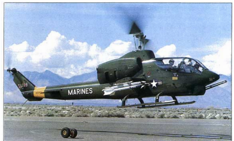
BuAer no. 159228 is a twin-engined AH-1J SeaCobra of the US Marine Corps, with the powerful General Electric M197 gun. It is seen on special trials at the Naval Weapons Center, China Lake, California, in March 1980. It was engaged in trials with AIM-9L Sidewinder self-defence AAMs, which were fired against target RPVs.
